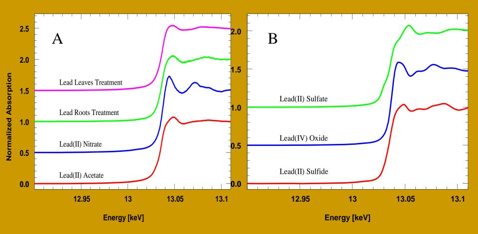
**A)** L<sub>III</sub> XANES of Pb-laden plant samples, lead(II) nitrate, and lead(II) acetate. LIII XANES of lead model compounds lead(II) sulfide, lead(II) sulfate, and lead(IV) oxide. **B)**
