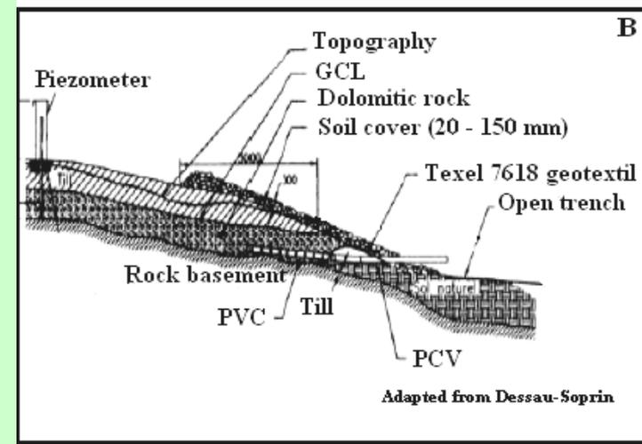
➤ Most of the dolomitic grains have a size between 26.5 and 37.5 mm, and the material does not contain particles finer than 7 mm.
