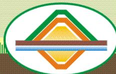
➤ Each drain consists of an isolated trench filled by dolomitic stones; A geosynthetic clay liner (GCL) was placed on top of each trench to ensure sealing.
